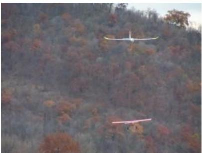
At release altitude, the flagging tape streamers help to visually confirm the separation of the Easy Glider Pro from the end of the towline.
