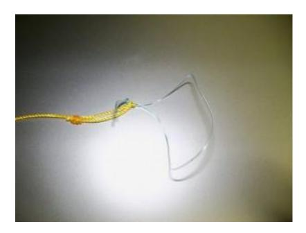
Loop this monofilament loop through one of the towline loops so that the knot end is located as pictured. This end will attach to the sailplane release.
