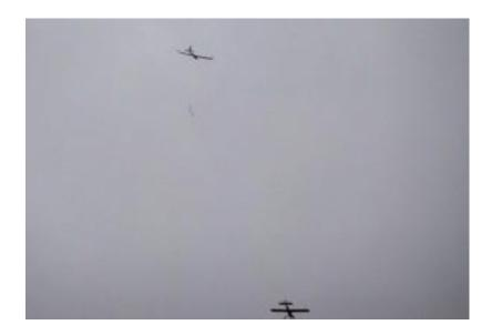
The flagging tape streamers also help the tow pilot see the end of the towline on landing.
