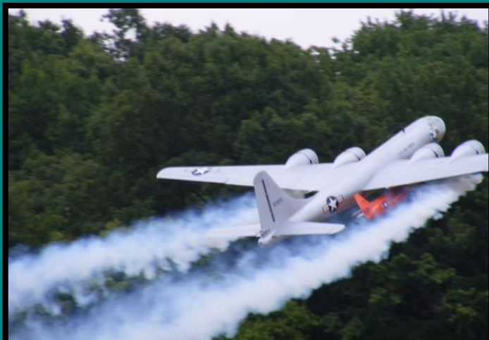
Mac Hodges' B29 taking off with "smoke on". Note the Bell X1 under the right wing. Once at altitude, Mac launches the X1, fires the rocket propulsion and after rocket burnout, another pilot glides the X1 back for a landing.
